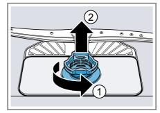
Pull down the micro filter to remove.
