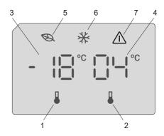
Once you have plugged in the product, all symbols will be displayed for 2 seconds and the initial values will be shown as -18 °C on the freezer adjustment indicator, and +4 °C on the fridge adjustment indicator.
