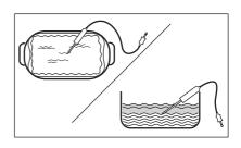
Step 4 Plug Food Sensor into the socket at the front of the oven.
