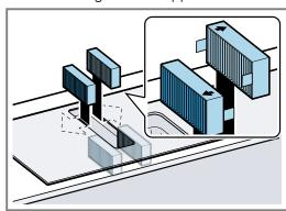
**5.** Insert the grease filter into the appliance.
