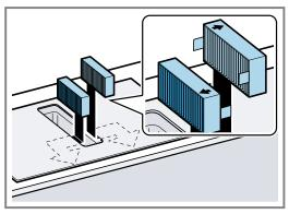
4. Insert the other odour filters or acoustics filters into the left and right of the appliance.
