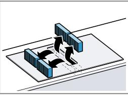
3. Insert two new odour filters or acoustics filters into the left and right of the appliance and slide them forwards.
