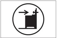
Install the anti-tilt protection B - 343 down from the top surface of the appliance and A - 67 mm from the side of the appliance into the circular hole on a bracket. Screw it into the solid material or use applicable reinforcement (wall).
