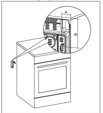
2. You can find the hole on the left side at the back of the appliance. Lift the front of the appliance and put it in the middle of the space between the cupboards. If the space between the bench cupboards is larger than the width of the appliance, you
