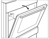
2. Hold the door trim (B) at the top edge of the door on both sides and push inwards to release the clip seal.
