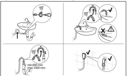
Make sure that the drain hose makes a loop to prevent particles going into the appliance from the sink.
