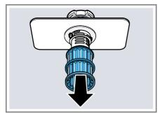
Press the locking catches ① together and lift the coarse filter out
