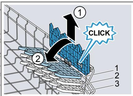
2. Position the etagere at a slight angle and move to the right height ②.
