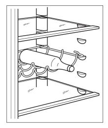
This shelf can be tilted to store unsealed bottles. To obtain this result, place front hooks of the shelf one level higher than the rear hooks.
