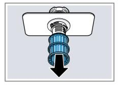
4. Press the locking catches 10 together and lift the coarse filter out ②.
