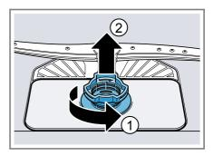
Pull down the micro filter to remove.
