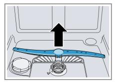
3. Check the outlet nozzles on the spray arms for blockages under running water and remove any foreign bodies.
