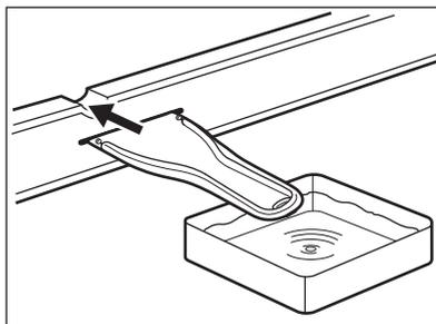
6. Dry the valve and slot in the rear wall:
