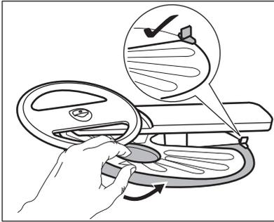
7. Reassemble the filters (B) and (C).
