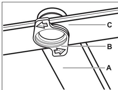
1. Release the stoppers on the sides of the sliding rails of the cutlery drawer and pull the drawer out.
