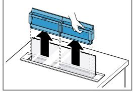
**3.** Insert the grease filter into the grease filter cart-ridges.
