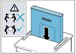
Insert the appliance evenly so that it is not tilted.Mark the cut-out for the pipework:
