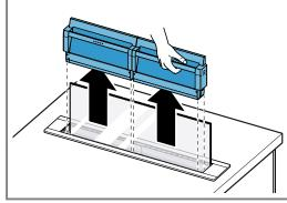
3. Remove the grease filters.
