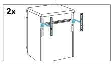
Undo and remove the screws on the horizontal transport strut.
