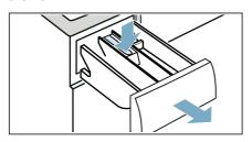
To remove the insert: Push the insert upwards from below with your finger.
