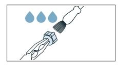
Connect the hose and check for leaks.
