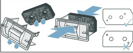
**Note:** Ensure that the filter mat is not misshapen, torn or clogged. Position the filter mat as shown above.
