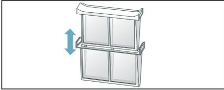
5. Open both filters and remove all the fluff.
