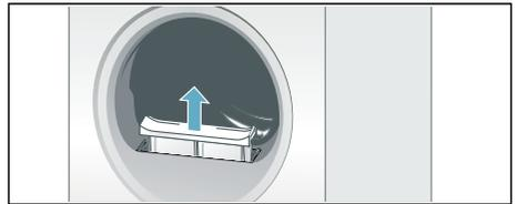
3. Remove the fluff from the recess in the fluff filter.
