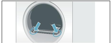
**Note:** Ensure that no fluff falls into the open shaft.
