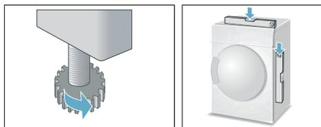
Incorrect alignment may cause high noise levels, vibrations and improper movement of the drum.
