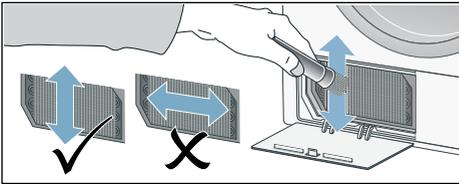
**Note:** Take care not to bend or damage the fins on the heat exchanger when cleaning it.
