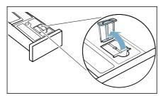
Remove the stopper inserted in the recess on the condensation container.
