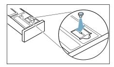
10. Pull the filter out of its snap-in lock.
