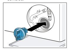
5. Insert the pump cap and screw it on as far as it will go.
