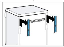
Undo and remove the screws in the horizontal transport strut using a T20 screwdriver.
