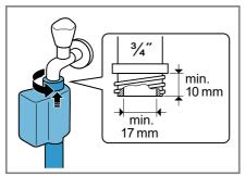
**2.** When connecting to a 21 mm =  $\frac{1}{2}$ " tap, first fit the adapter with a sealing washer.
