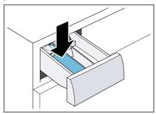
To prevent foaming, use only half of the amount of detergent recommended by the detergent manufacturer for light soiling. Do not use detergent suitable for woollens or delicates.
