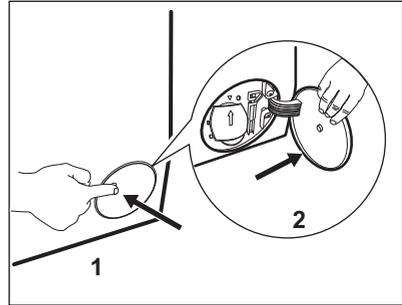
2. Place a suitable bowl below the drain pump access to collect the water that flows out.
