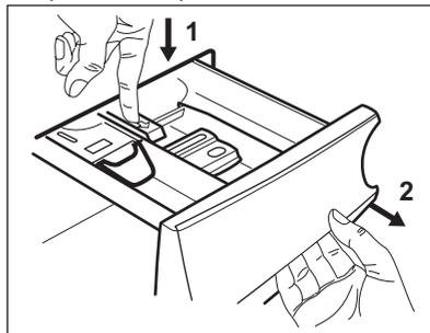
2. Remove the top part of the additive compartment to aid cleaning and flush it out under running warm water, to remove any traces of accumulated detergent. After cleaning, replace the top part in its position.
