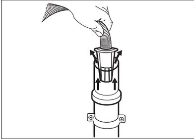
5. **Without the plastic hose guide, to a sink spigot** - Put the drain hose in the spigot and tighten it with a clamp. Refer to the illustration.
