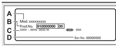
The rating plate reports the model name (A), product number (B), electrical ratings (C) and serial number (D).
