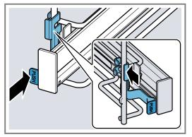
2. Press and hold **PUSH** ① and swing the rail outwards ② until the front retainer ⓐ is detached.
