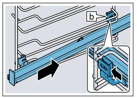
**3.** Press and hold **PUSH** ① and swing the pull-out rail inwards ② until the retainer ⓐ is attached in the lower rod.
