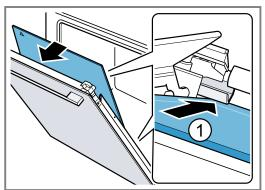
Note: The intermediate pane is automatically positioned by the rotational movement of the spacer. Slide the second intermediate pane into the central retainer ① and fit it at the top.
