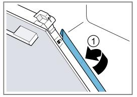
**4.** Note: The lettering "Pyro" must be legible at the top, as shown in the picture.
