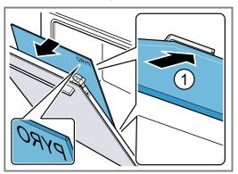
Push the inner pane in at the top ①. Push the sliding caps a downwards in the direction of the arrow.
