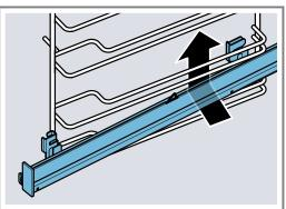
Guide the rail lengthways to the rear to the guide rods, and slide both retainers onto each lower rod. In doing so, use the rear retainer b to grip the vertical rod.
