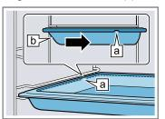
**3.** To place the accessory at shelf positions with pullout rails, pull out the pull-out rails. Wire rack or baking tray Place the accessory so that it is inserted on the rear stop of the pull-out system.
