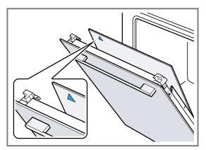
1. Slide the first intermediate pane into the lowest retainer ① and fit it at the top.
