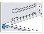
**Note:** The pull-out rails lock in place when they are fully pulled out. Gently push the pull-out rails back into the cooking compartment.
