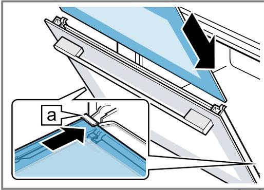
When doing this, ensure that the smooth, glossy side of the panel is on the outside and the cut-outs on the left and right are at the top. The panel must be sitting correctly at the bottom in the retainer.
