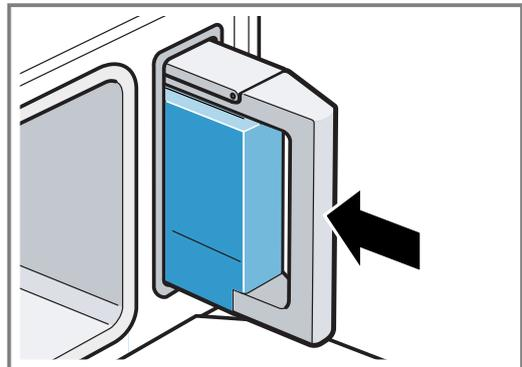
7. Check that the water tank is flush with the water tank recess.
