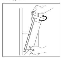
To remove the glass cover of the ExtraZone compartment:
