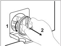
6. Turn the filter anti-clockwise to remove it
