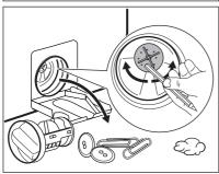
7. If it is necessary, remove fluff and objects from the filter recess.
