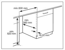
This appliance has been designed to be built into the kitchen furniture. See the minimum recess dimensions in the drawings.
