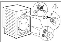
**6.** Remove the three bolts, the hose holders and plastic spacers by using the spanner supplied with the appliance.
