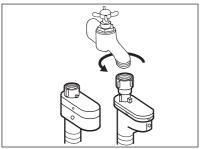
**5.** Connect the water inlet hose to the cold water tap with 3/4 thread.
