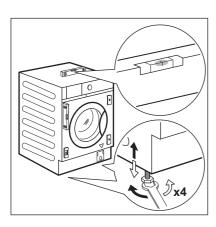
1. Install the appliance on a flat hard floor.
