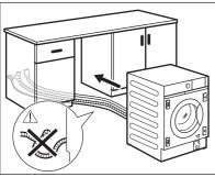
Before proceeding with appliance building in, bring it near the recess and preposition the inlet hose, the drain hose and the mains cable.
