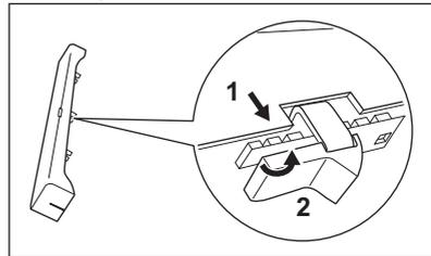
4. Hold the door trim B at each side and position it on the inner edge of the door. Put the door trim into the top edge of the door.
