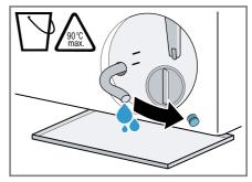
8. Firmly press on the sealing cap.
