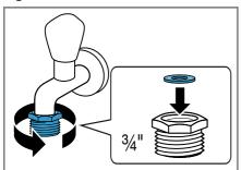
Open the water tap carefully and check that the connection points are tight.
