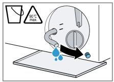
8. Firmly press on the sealing cap.
