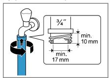
**3.** When connecting to a 21 mm =  $\frac{1}{2}$ " tap, first fit the adapter with a sealing washer.
