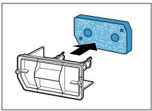
Ensure that you do not deform or damage the filter mat.
