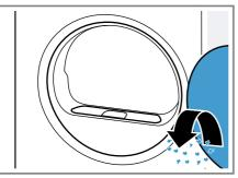
3. Remove the two-part fluff filter.
