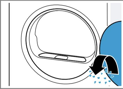
3. Remove the two-part fluff filter.
