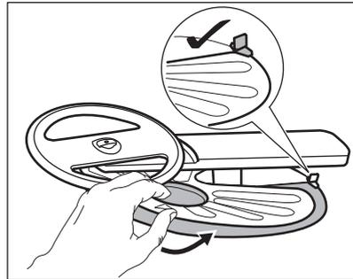
7. Reassemble the filters (B) and (C).
