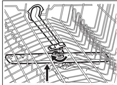
3. Wash the spray arm under running water. Use a thin pointed tool, e.g. a toothpick, to remove particles of soil from the holes.
