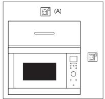
The electrical outlet should be readily accessible so that the unit can be unplugged easily in an emergency. Or it
