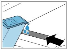
Observe the mark for filling the water tank next to the front opening. If ♠ does not go out on the display, align the appliance correctly.
