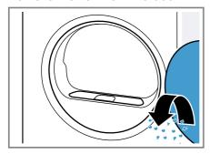
3. Remove the two-part fluff filter.
